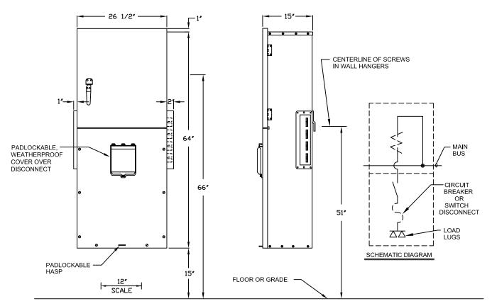
NOTES: END COVERS ARE REMOVABLE, & ARE TO BE INSTALLED ON END UNITS USING CARRIAGE BOLTS TO PREVENT UNAUTHORIZED ACCESS TO BUS BARS.
